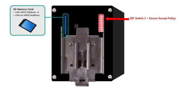
Position of the DIP switch on 16XX Industrial switches:
