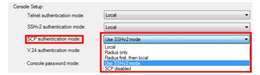
In addition, it is possible to create an "IP Access-List" to authorize only certain IP addresses or a range of IP addresses which are allowed to access to the SCP server.
