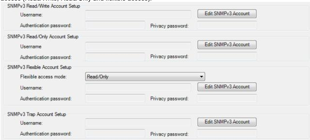
The passwords for the authentication and the encryption can be configured separately.
